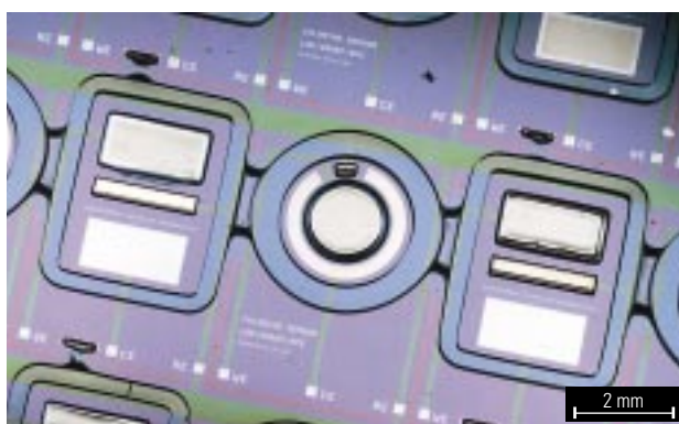
Integrated Electrochemical Sensor, Amperometric Sensor device on 4" silicon wafers
